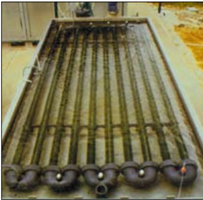
6.23. Continuous loop photobioreactor (Courtesy of L. Tomaselli 1 ).
