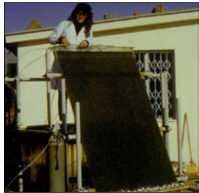
6.23. Continuous loop photobioreactor (Courtesy of L. Tomaselli 1 ).
