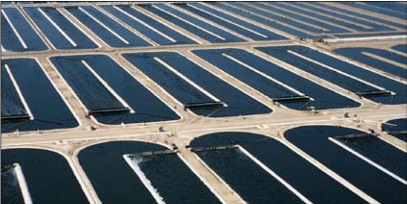
6.5. Primary production ponds have food grade liners. Each pond is 5000 square meters- larger than a football field.
