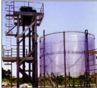
6.25. Commercial tubular photobioreactor (Courtesy of Microalgae Spa Italy 3 ).
